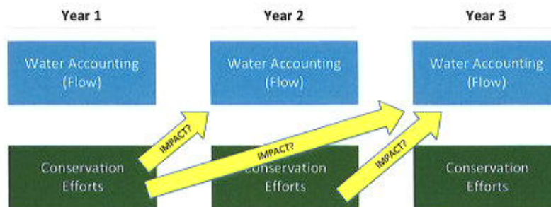
Figure 5. Conservation efforts in one year can affect water use in future years. If reasonable data can be gathered, water losses isolated, and weather and population normalized, one can measure the accumulated impact of conservation over time.
